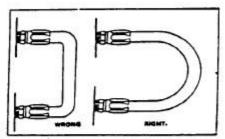
At bends, provide enough hose for a wide radius curve. Too tight a bend pinches the hose and restricts the flow. The line could even kink and close entirely. In many cases, use of the right fittings or adapters can eliminate bends or kinks.
