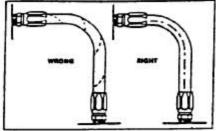
If a hose is installed with a twist in it, high operating pressures tend to force it straight. This can loosen the litting nut. Twisting can cause reinforcement separation and the hose could burst at the point of strain.
