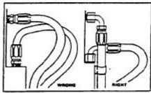
Use elbows and adapters in the installation to relieve strain on the assembly, and to provide easier and nester installations that are accessible for inspection and maintenance. Remember that metal and fittings cannot be considered as part of the flexible portion of the assembly.
