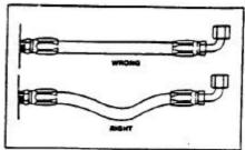
Under pressure, a hose may change in length. Always provide some stack in the hose to allow for this shrinkage or expansion. (However, excessive stack in hose lines is one of the most common causes of poor appearance.)
